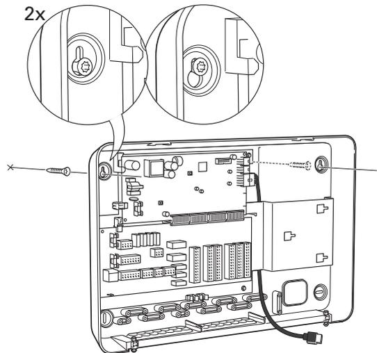
6. Refit the display. Screw SMO S40 into place at the lower edge with the two remaining screws.
