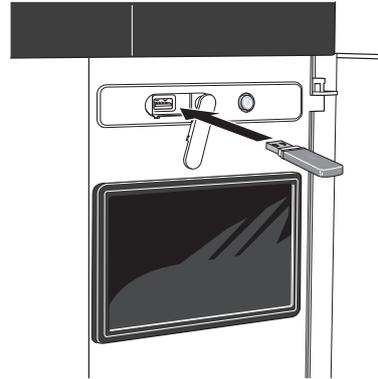
When a USB memory is connected, a new menu (menu 8) appears in the display.
