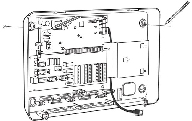
5. Hook SMO S40 onto the screws on the wall.
