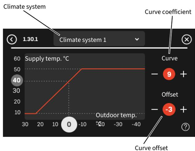
1. Select the climate system (if more than one) for which the curve is to be changed.
