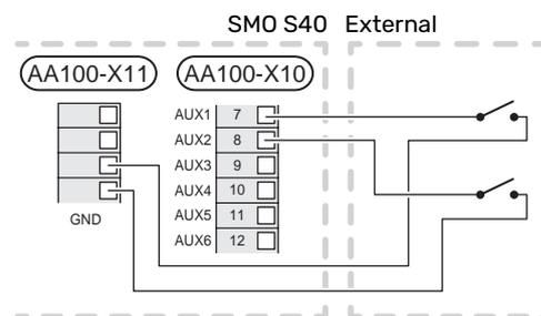
The example above uses the inputs AUX1 (AA100-X10:7) and AUX2 (AA100-X10:8).
