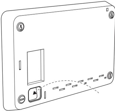
3. Remove the display by moving it to the left. Detach the cable from the lower edge
