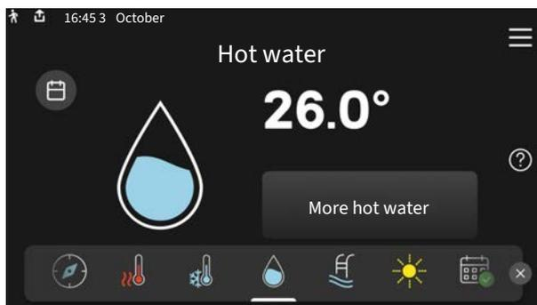
Here, you can start or stop a temporary increase in the hot water temperature.
