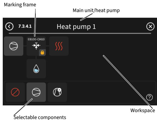
*Main unit/heat pump:* Here, you select the heat pump for which the docking setting is to be made (if the heat pump is solitary in the system, only the main unit is shown).
