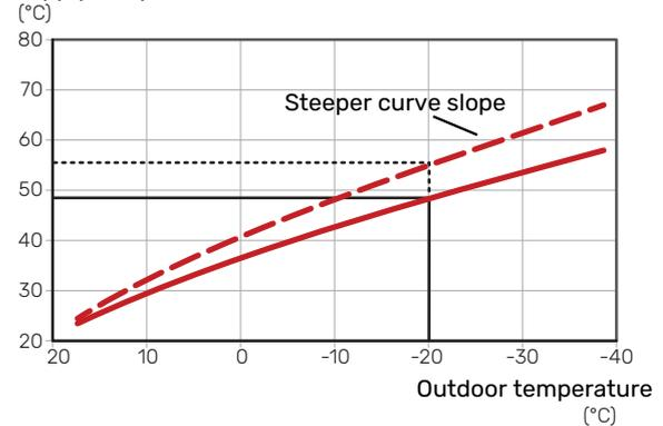
The optimum curve slope depends on the climate conditions and the lowest dimensioned outdoor temperature (DOT) in your location, whether the house has radiators, fan coils or underfloor heating and how well insulated the house is.
