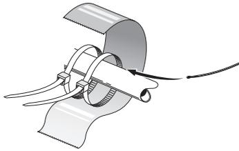
The temperature sensors are fitted using heat conducting paste, cable ties (the first cable tie is secured to the pipe in the middle of the sensor and the other cable tie is mounted approx. 5 cm after the sensor) and aluminium tape. Then insulate them using the enclosed insulation tape.
