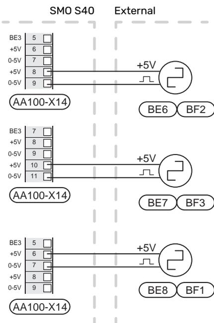
Activate the meter(s) in menu 7.2 - "Accessory settings" and then set the desired value ("Energy per pulse" or "Pulses per kWh") in menu 7.2.19 - "Pulse energy meter".
