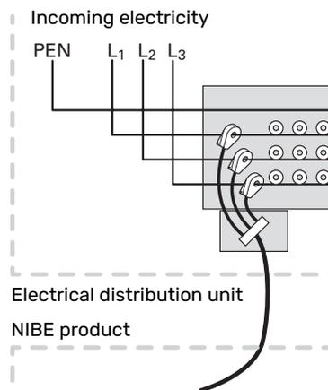
3. Connect the sensor to terminal block AA100-X14:BE1-BE3 and to any terminal block on AA100-X13:GND.
