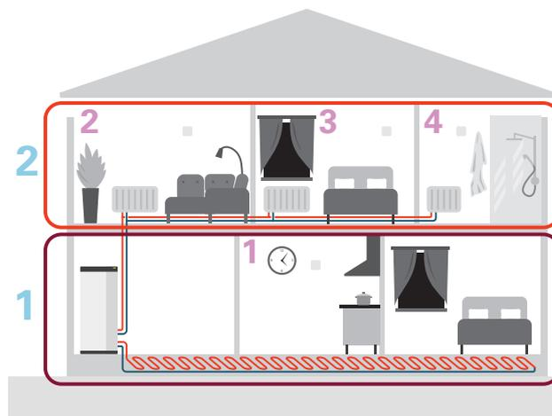
This example shows a property with two climate systems (1 and 2, two separate floors) divided into four zones (1-4, four different rooms). The temperature can be controlled individually in each zone (accessory required).
