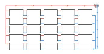
If a double sided Tichelmann connection is not an option, it is possible to do a single-sided Tichelmann connections. A double-sided connection will always have better flow characteristics.
