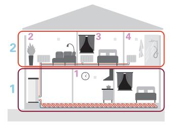
This example shows a property with two climate systems (1 and 2, two separate floors) divided into four zones (1-4, four different rooms). Temperature and demand-controlled ventilation can be controlled individually for each zone (accessory required).
