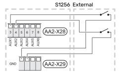
The example above uses the inputs AUX1 (AA2-X28:3) and AUX2 (AA2-X28:4).
