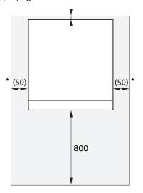
\* A normal installation needs 300 – 400 mm (any side) for connection equipment, e.g. level vessel, valves and electrical equipment.
