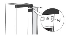
2. Pull the panel's top edge towards you and lift diagonally upwards to remove it from the frame.
