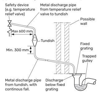
If the vertical section, 300 mm, is difficult to fill, there is a vertically adjustable bracket as an accessory.
