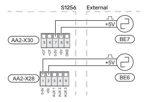
Activate the meter(s) in menu 7.2 - "Accessory settings" and then set the desired value ("Energy per pulse" or "Pulses per kWh") in menu 7.2.19 - "Pulse energy meter".
