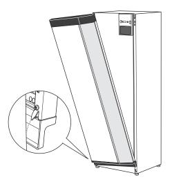
4. Press the top of the front section against the frame and screw it into place.
