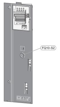
The temperature limiter (FQ10) cuts the power supply to the electric additional heat if the temperature rises above 89 °C and it is reset manually.
