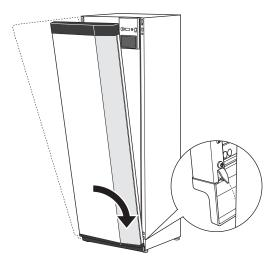
3. Check the display is straight. Adjust if necessary.
