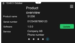
Here, you can find information about product name, the product's serial number, the version of the software and service. When there is new software to download, you can do it here (provided that S1256 is connected to myUplink).
