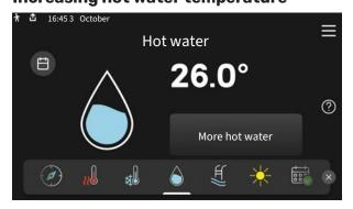
Here, you can start or stop a temporary increase in the hot water temperature.  $\,$
