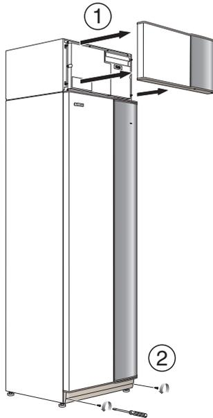
3. Lift the panel out at the bottom edge and up.
