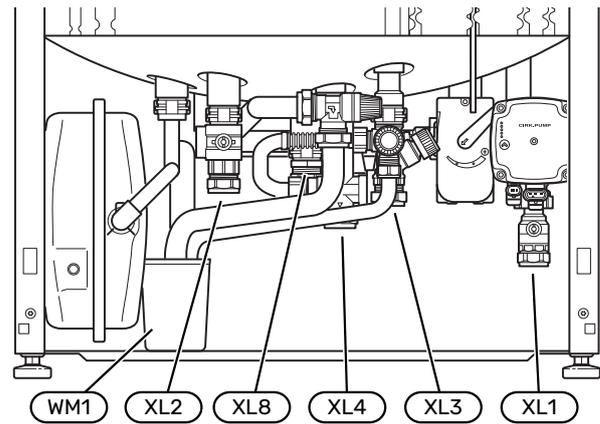
The overflow cup (WM1) can be turned, allowing the pipe to be pointed forwards or backwards to simplify connection to the drain.
