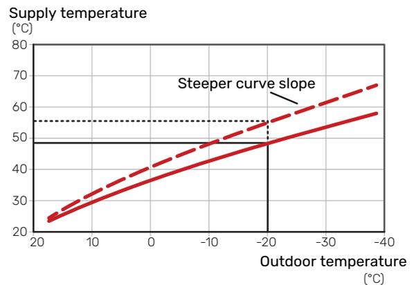
The optimum curve slope depends on the climate conditions and the lowest dimensioned outdoor temperature (DOT) in your location, whether the house has radiators, fan coils or underfloor heating and how well insulated the house is.
