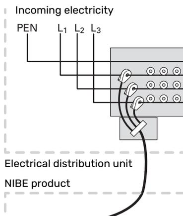
3. Connect the cable to the input board (AA3) on terminal block X4:1-4 where X4:1 is the common terminal block for the three current sensors.
