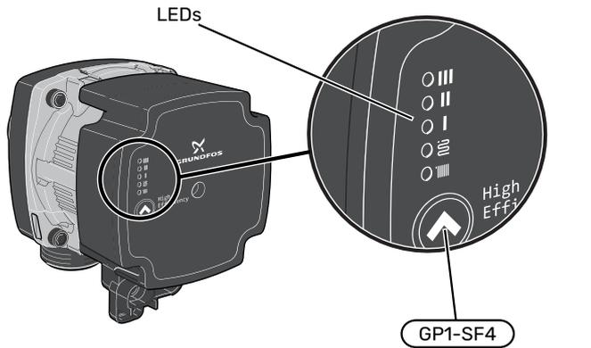
The circulation pump (GP1) is equipped with five LEDs. In normal mode, the LEDs show the pump's setting by lighting up in green and/or yellow. The LEDs can also indicate an alarm, in which case they light up in red and yellow.
