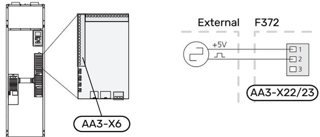
Activate the energy meter(s) in menu 5.2.4 and then set the desired value (energy per pulse) in menu 5.3.21.
