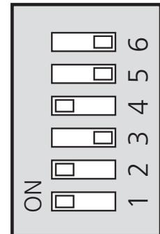
The image shows the dip-switch (AA1-S2) in the factory setting.
