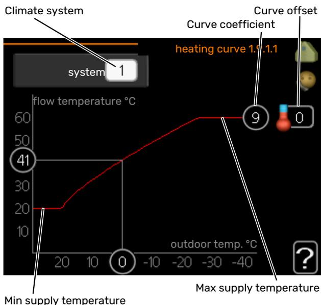
1. Select the climate system (if more than one) for which the curve is to be changed.
