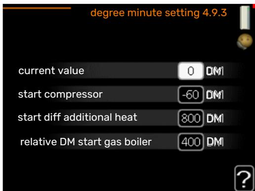
Degree minutes are a measurement of the current heating requirement in the house and determine when the compressor respectively additional heat will start/stop.
