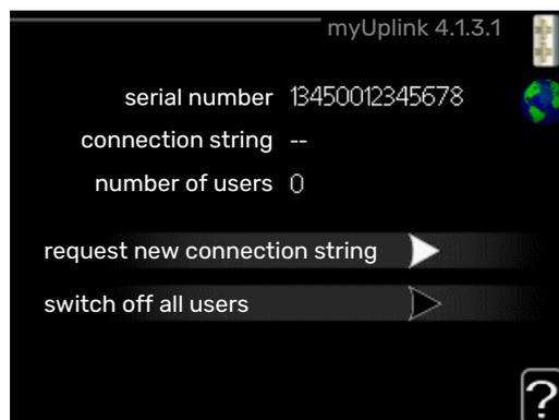
Here you can manage the installation's connection to myUplink (myuplink.com) and see the number of users connected to the installation via the internet.
