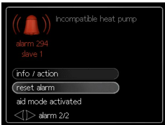
In the event of an alarm with a red status lamp a malfunction has occurred that the heat pump and/or control module cannot remedy itself. In the display, by turning the control knob and pressing the OK button, you can see the type of alarm it is and reset it. You can also choose to set the installation to aid mode.
