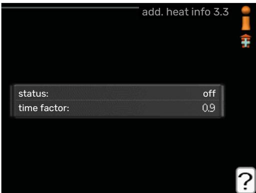
Information about the additional heat's settings, operating status and statistics can be obtained here. No changes can be made. The information is on several pages. Turn the control knob to scroll between the pages.
