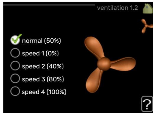
The ventilation in the accommodation can be temporarily increased or reduced here.
