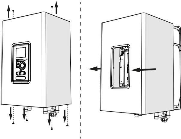
1. Unscrew the bolts from the lower edge of the front cover.
