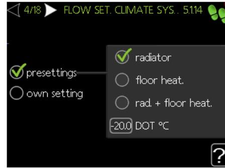
DOT = Design Outdoor temperature. Set here a temperature which is the lowest outdoor temperature in the winter used for designing the building and installation (depends of the land or region where the heat pumps will be installed).
