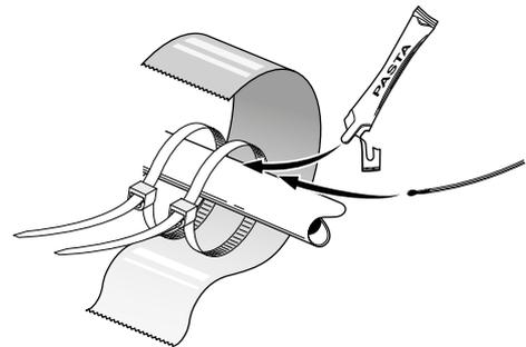
The temperature sensors are fitted using heat conducting paste, cable ties (the first cable tie is secured to the pipe in the middle of the sensor and the other cable tie is mounted approx. 5 cm after the sensor) and aluminium tape. Then insulate them using the insulation tape.
