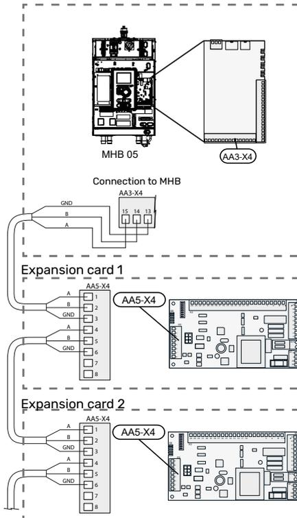
For detailed information on using the expansion card, see the installer manual for the AXC 40 accessory. The connections 13-14-15 on AA3-X4 can be used both for communication with the outdoor unit and an AA5 card.
