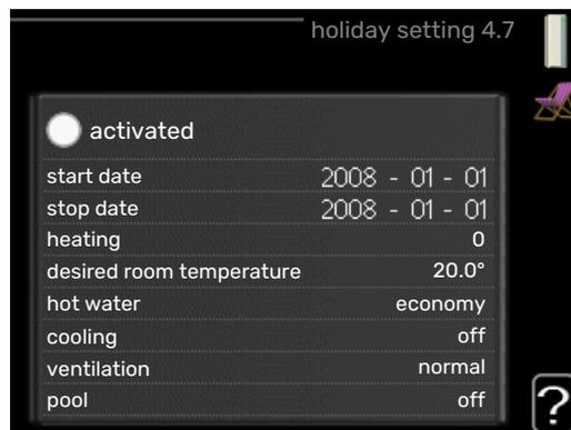
To reduce energy consumption during a holiday you can schedule a reduction in heating and hot water temperature. Cooling, ventilation, pool and solar panel cooling can also be scheduled if the functions are connected.
