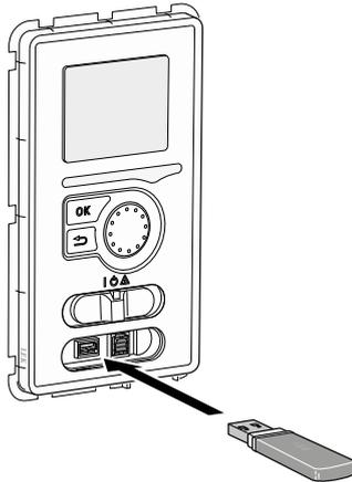
The display unit is equipped with a USB socket that can be used to update the software, save logged information and manage the settings in the controller.
