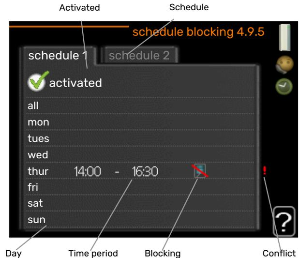
The additional heat can be scheduled to be blocked for up to two different time periods here.
