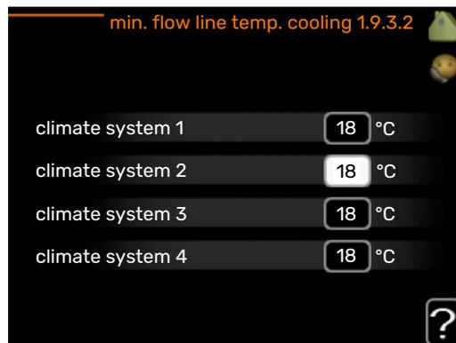
In menu 1.9.3 you select heating or cooling, in the next menu (min. supply temp.heating/cooling) set the minimum temperature on the supply temperature to the climate system. This means that MHB 05 never calculates a temperature lower than that set here.
