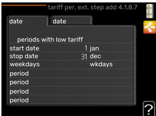
Here you can use tariff control for the external step controlled additional heat.
