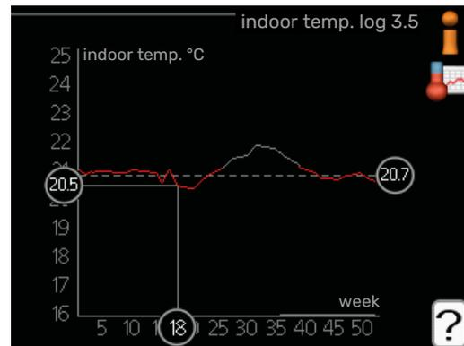
Here you can see the average temperature indoors week by week during the past year. The dotted line indicates the annual average temperature. The average outdoor temperature is only shown if a room temperature sensor/room unit is installed.
