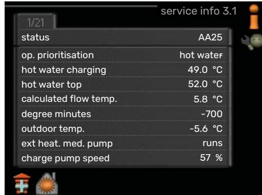
Information about the actual operating status of the installation (e.g. current temperatures etc.) can be obtained here. No changes can be made.
