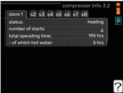
Information about the compressor's operating status and statistics can be obtained here. No changes can be made. The information is on several pages. Turn the control knob to scroll between the pages.
