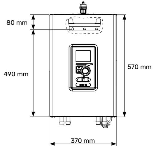
1. Place the included mounting hanger horizontally against the wall. Level the hanger using the spirit level. Mark the points for the mounting holes to be drilled.
