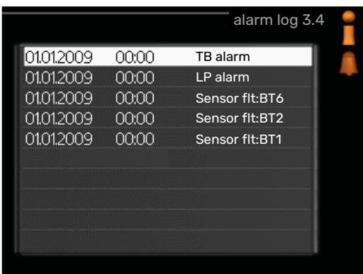
To facilitate troubleshooting, the installation's operating status at alarm alerts is stored here. You can see information for the 10 most recent alarms. To view the run status in the event of an alarm, mark the alarm and press the OK button.
