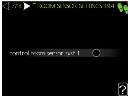
In case an on/off room thermostat is connected, do not enable this option.
