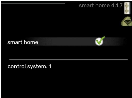
When you have a smart home system that can speak to myUplink, by activating the smart home function in this menu you can control the MHB 05 via an app.
