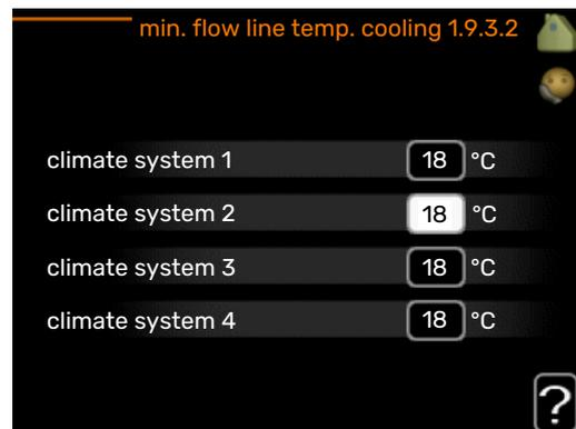
In menu 1.9.3 you select heating or cooling, in the next menu (min. supply temp.heating/cooling) set the minimum temperature on the supply temperature to the climate system. This means that F1345 never calculates a temperature lower than that set here.
