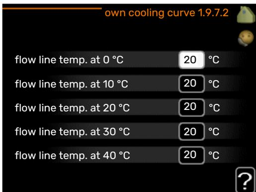
When required, create your own heating or cooling curve here, by setting the desired supply temperatures for different outdoor temperatures.
