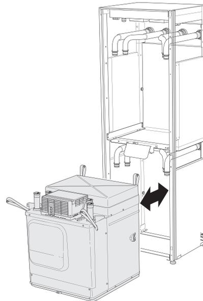
If the heat pump is not secured in position the upper cooling module must always be removed before the lower one can be pulled out.
