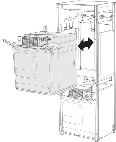
9. Carefully pull out the lower cooling module (EP14) using the module's lifting eyes.
