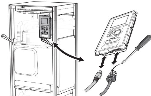
7. Remove the two screws holding the display unit in the frame (this procedure only needs to be done if you are going to pull out the upper cooling module).
