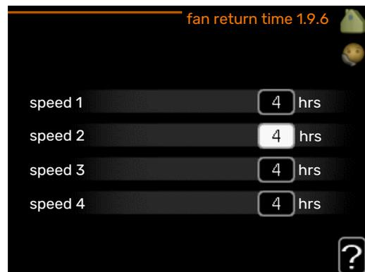
Here you select the return time for temporary speed change (speed 1-4) on the ventilation in menu 1.2.
