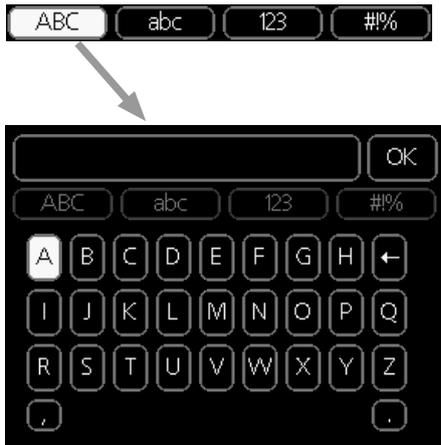
Depending on the menu, you can gain access to different character sets which you can select using the control knob. To change character table, press the Back button. If a menu only has one character set the keyboard is displayed directly. When you have finished writing, mark "OK" and press the OK button.
