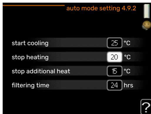
When the operating mode is set to "auto", the heat pump selects when start and stop of additional heat and heat production is permitted, dependent on the average outdoor temperature. If accessories for cooling are present or if the heat pump has the integrated cooling function, you can also select the start temperature for cooling.
