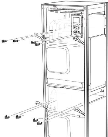
6. Remove the connector from the underside of the display unit (this procedure need only be done if you are going to pull out the upper cooling module).
