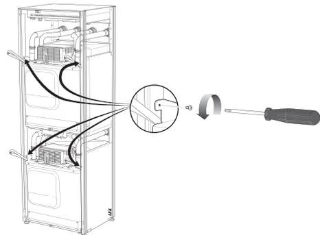
5. Pull off the clips (four for each cooling module) and separate the pipes carefully.
