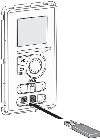
The display unit is equipped with a USB socket that can be used to update the software and save logged information in F1345.
