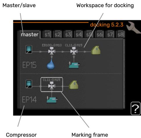
**Master/slave:** Select the heat pump for which the docking setting is to be made (if there is only one heat pump in the system, only master is displayed).
