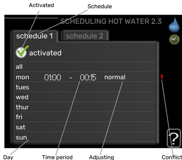
What hot water comfort the heat pump is to work with can be scheduled here for up to two different time periods per day.
