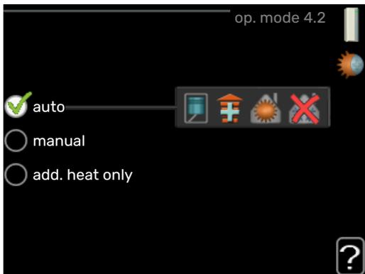
The heat pump operating mode is usually set to "auto". It is also possible to set the heat pump to "add. heat only", but only when an addition is used, or "manual" and select yourself what functions are to be permitted.
