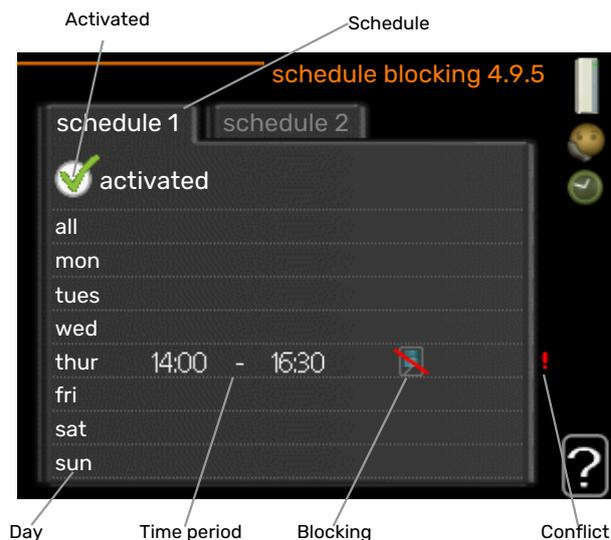
The compressors in the heat pump and/or connected additional heating can be scheduled to be blocked for up to two different time periods here. If several heat pumps are connected as master/slave their compressors are blocked as well.
