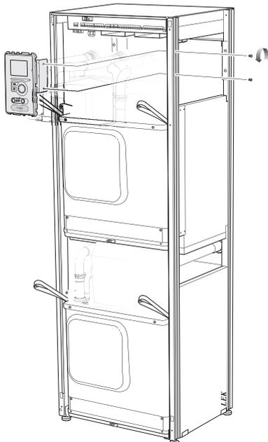
8. Carefully pull out the upper cooling module (EP15) using the module's lifting eyes.
