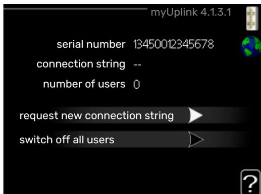
Here you can manage the installation's connection to myUplink (<http://www.nibeuplink.com>) and see the number of users connected to the installation via the internet.
