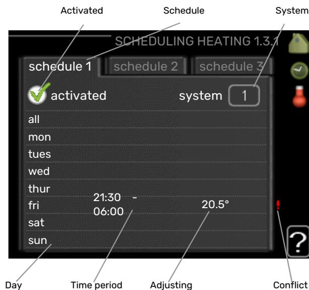
Increases or decreases in the accommodation temperature can be scheduled here for up to three time periods per day. If a room sensor is installed and activated the desired room temperature (°C) is set during the time period. Without an activated room sensor the desired change is set (of setting in menu 1.1). One step is usually enough to change the room temperature by one degree, but in some cases several steps may be required.
