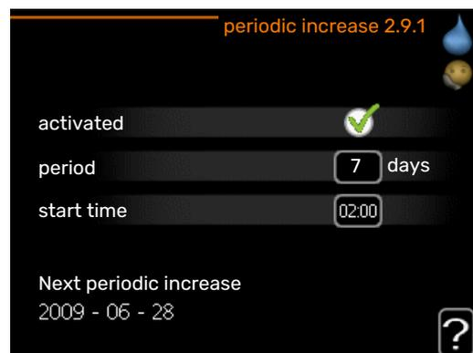
To prevent bacterial growth in the water heater, the compressor and the immersion heater can increase the hot water temperature for a short time at regular intervals.
