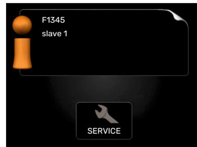
If the heat pump is set as slave a limited main menu is displayed because the majority of the settings for the system are made at the master heat pump.
