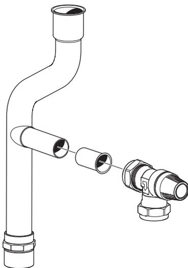
3. Then fit the safety valve with the associated pipes. The safety valve must be at an angle of 45°. Fit the clip. Twist the clip to ensure that it fastens properly.
