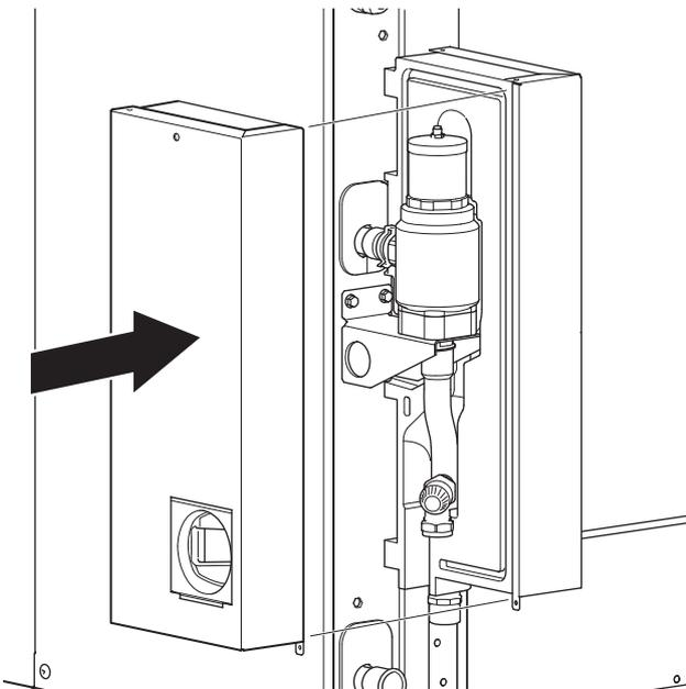
8. Fit the cover. Secure with three screws. Two screws in the lid, on the right and left-hand sides, and one screw in the bottom.
