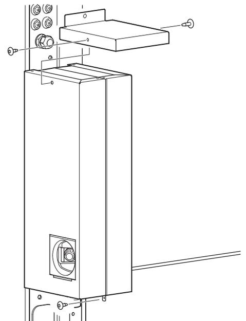
9. Secure the gas separator to the heat pump using two screws, one at the top and one at the bottom.
