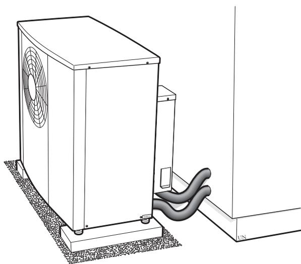
All outdoor pipes must be insulated with at least 19 mm thick pipe insulation.
