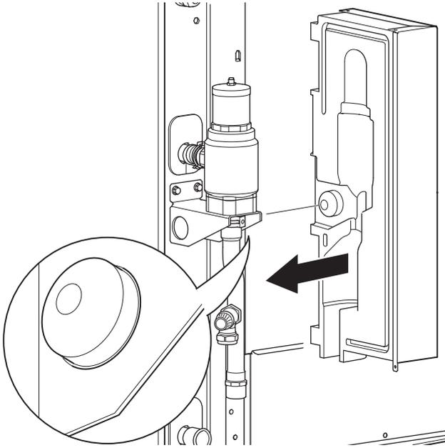
7. Check that both halves of the gas separator are properly in place, parallel with the edge of the heat pump.
