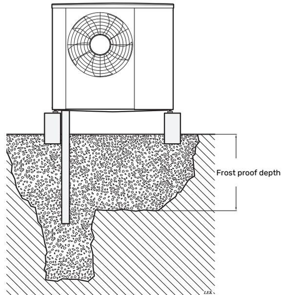
If the house has a cellar the stone caisson must be positioned so that condensation water does not affect the house. Otherwise the stone caisson can be positioned directly under the heat pump.
