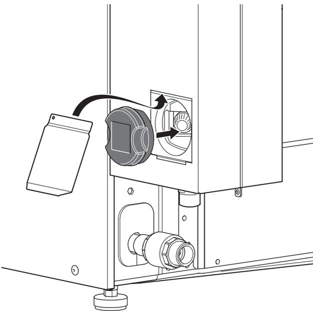
11. Screw the flexible pipes into place. The flexible pipes can be installed angled straight back or down, depending on which of the pipe connections the 90° bend is in-
