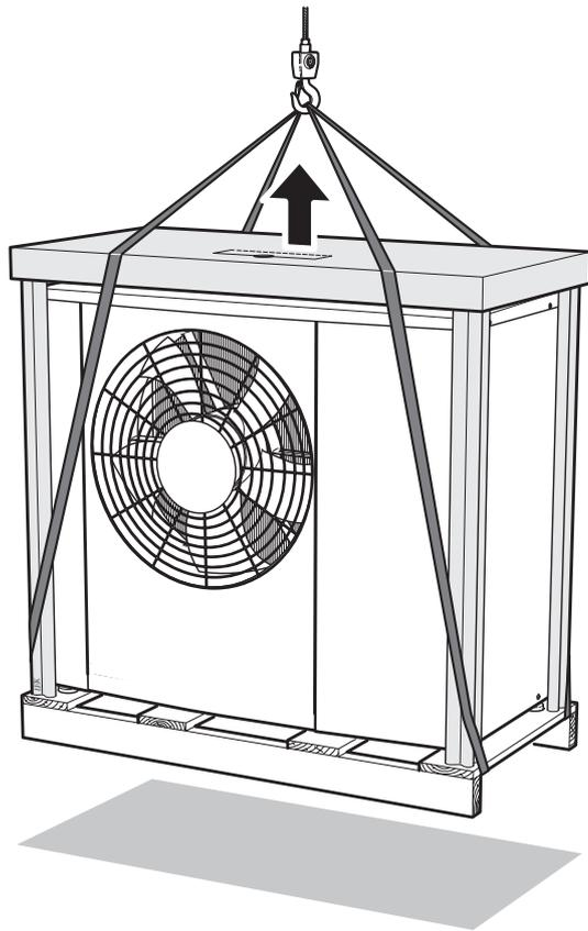
If the heat pump needs to be transported across soft ground, such as a lawn, we recommend using a crane truck that can lift it to the installation location. When the heat pump is lifted with a crane, the packaging must be intact.
