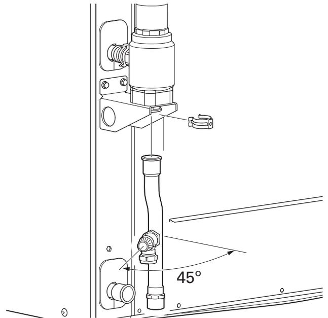
4. Install the non-return valve. Fit the clip. Twist the clip to ensure that it fastens properly.
