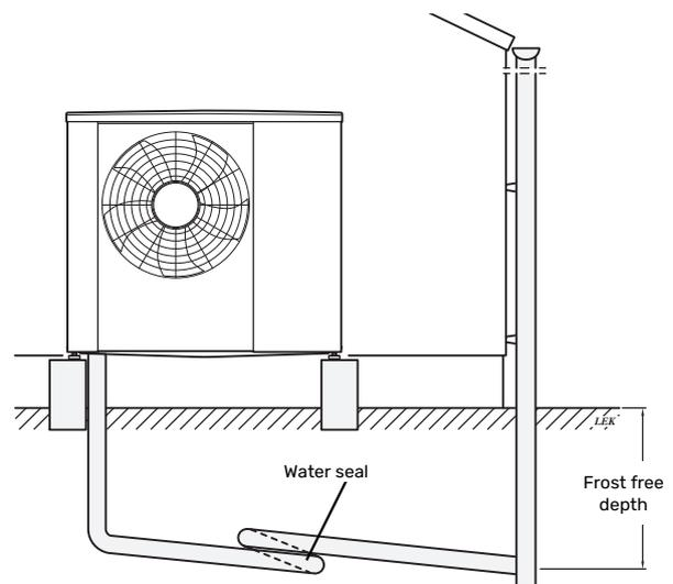
Route the pipe sloping down from the heat pump. The condensation water pipe must have a water seal to prevent air circulation in the pipe.
