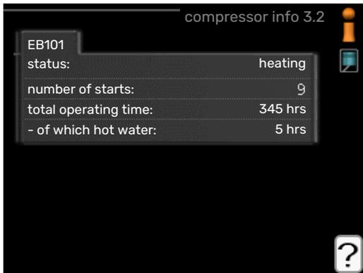
Information about the compressor's operating status and statistics can be obtained here. No changes can be made.
