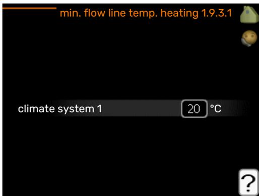
In menu 1.9.3 you select heating or cooling, in the next menu (min. supply temp.heating/cooling) set the minimum temperature on the supply temperature to the climate system. This means that SMO 20 never calculates a temperature lower than that set here.
