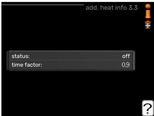
Information about the additional heat's settings, operating status and statistics can be obtained here. No changes can be made.
