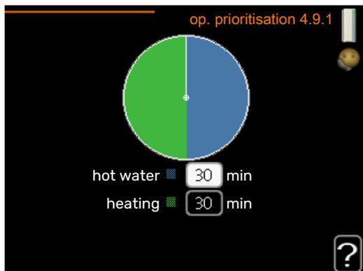
The indicator marks where in the cycle the installation is.
