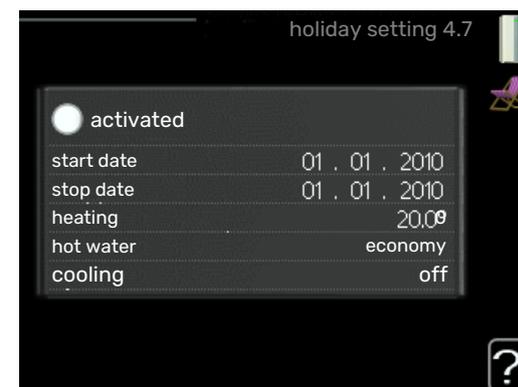
If a room sensor is installed and activated, the desired room temperature (°C) is set during the time period.
