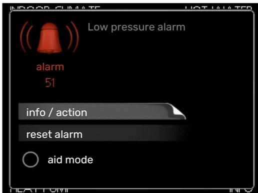
In the event of an alarm, some kind of malfunction has occurred, which is indicated by the status lamp changing from green continuously to red continuously. In addition, an alarm bell appears in the information window.
