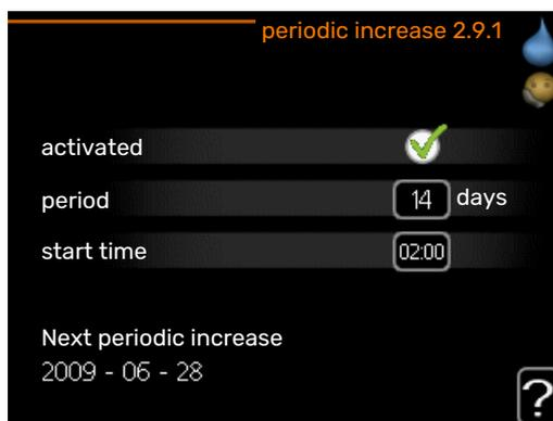
To prevent bacterial growth in the water heater, the heat pump and any additional heater can increase the hot water temperature for a short time at regular intervals.
