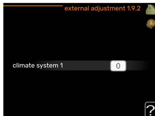
Connecting an external contact, for example, a room thermostat or a timer allows you to temporarily or periodically raise or lower the room temperature while heating. When
