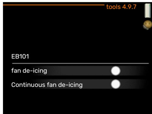
This function ensures that any ice on the fan or fan grille is removed.
