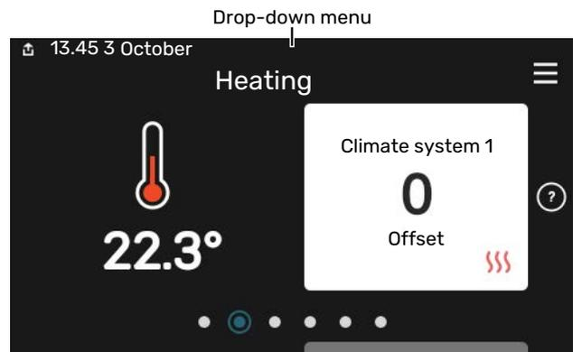
The drop-down menu shows the current status for VVM S330, what is in operation and what VVM S330 is doing at the moment. The functions that are in operation are highlighted with a frame.
