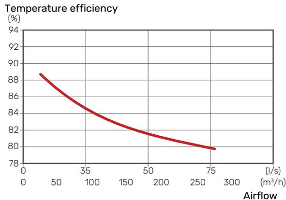
Outdoor air: 5 °C Exhaust air 25 °C RH exhaust air: <27.7 %
