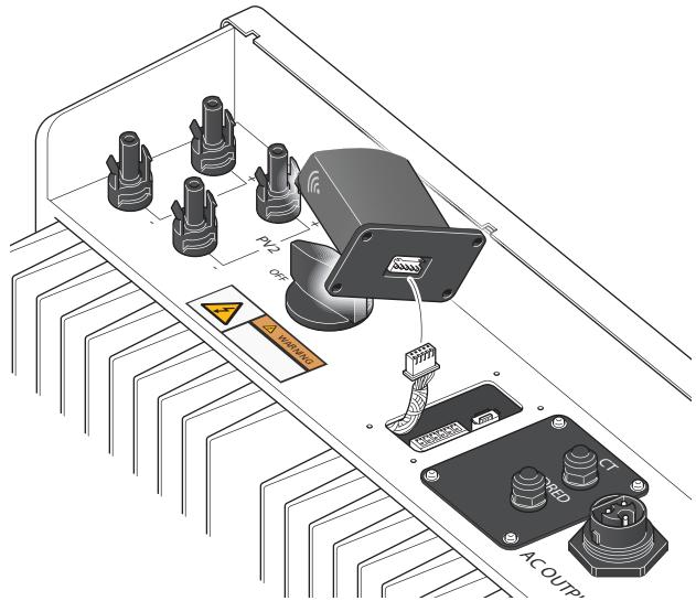
4. Screw the communication module into place, checking that the cable is properly located before you screw it in place.
