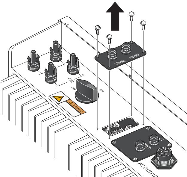
3. Pull out the white cable and install it in the communication module. It may be hidden under the edge, so carefully ease it out. It is connected at one end, so pull it out carefully and connect it to CMO 11.
