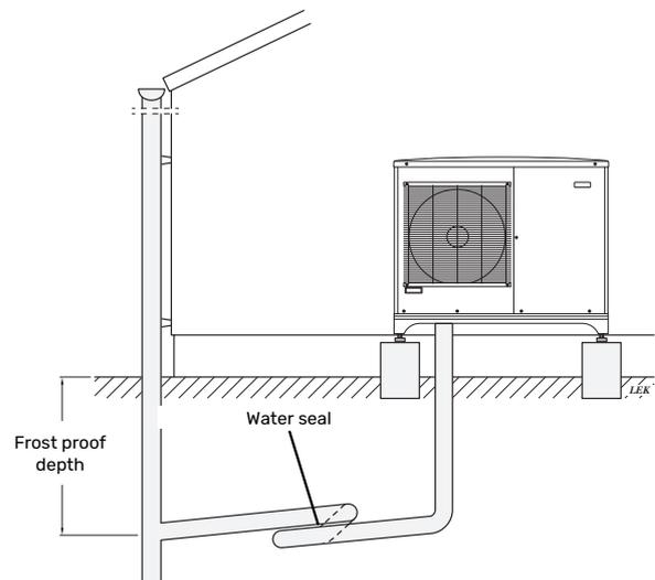
Route the pipe sloping downward from the heat pump. The condensation water pipe must have a water seal to prevent air circulation in the pipe.
