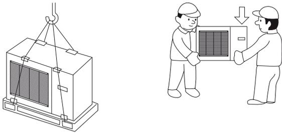
If the heat pump needs to be transported across soft ground, such as a lawn, we recommend using a crane truck that can lift it to the installation location. When the heat pump is lifted with a crane, the packaging must be intact.
