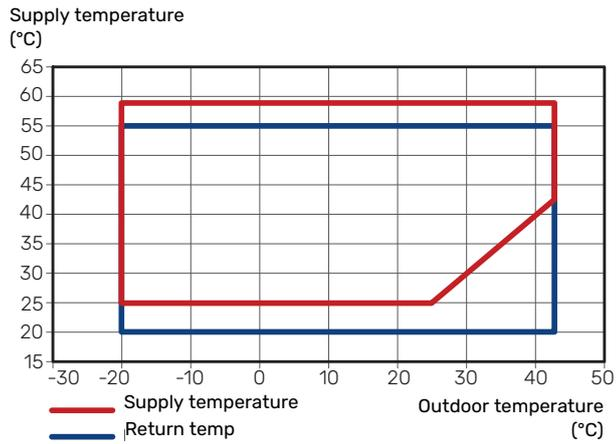
The supply temperature is permitted to be lower for a short period, e.g. at start-up.
