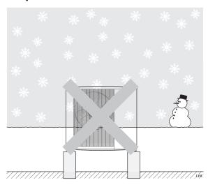
Prevent snow from building up and covering the grilles and drain holes on F2120.
