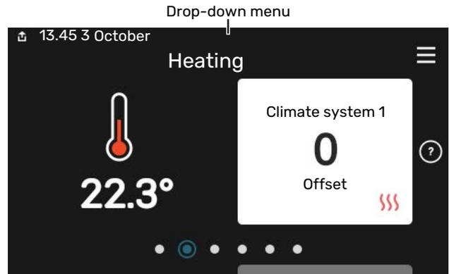
The drop-down menu shows the current status for SMO S40, what is in operation and what SMO S40 is doing at the moment. The functions that are in operation are highlighted with a frame.
