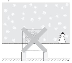
Prevent snow from building up and covering the grilles and drain holes on S2125.
