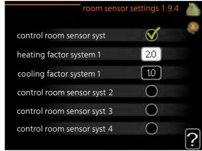
Room sensors to control the room temperature can be activated here.
