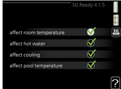
With low price mode on "SG Ready" the parallel offset for the indoor temperature is increased by "+1". If a room sensor is installed and activated, the desired room temperature is instead increased by 1 °C.
