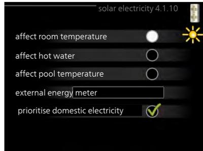
This is where you set which part of your installation (room temperature, hot water temperature, pool temperature) is to benefit from the solar electricity surplus.
