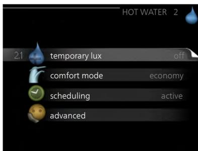
**temporary lux** Activation of temporary increase in the hot water temperature. Status information displays "off" or what length of time of the temporary temperature increase remains.
