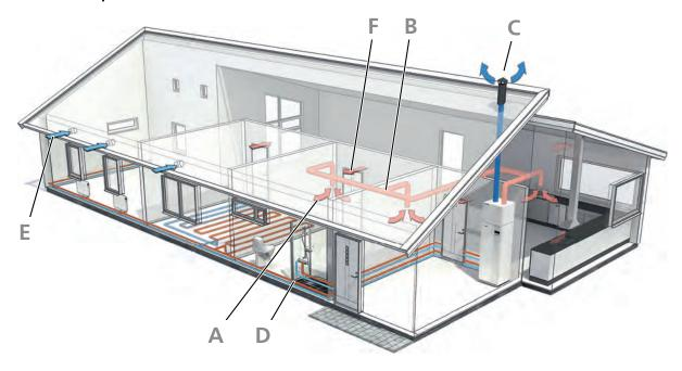
F750 is an exhaust air heat pump with integrated fan and a water heater provided with corrosion protection in the form of copper, enamel or stainless steel. There is an integrated immersion heater used as an additional heater when it becomes really cold outside.
