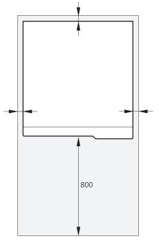
Ensure that there is sufficient space (300 mm) above F750 for installing ventilation hoses.
