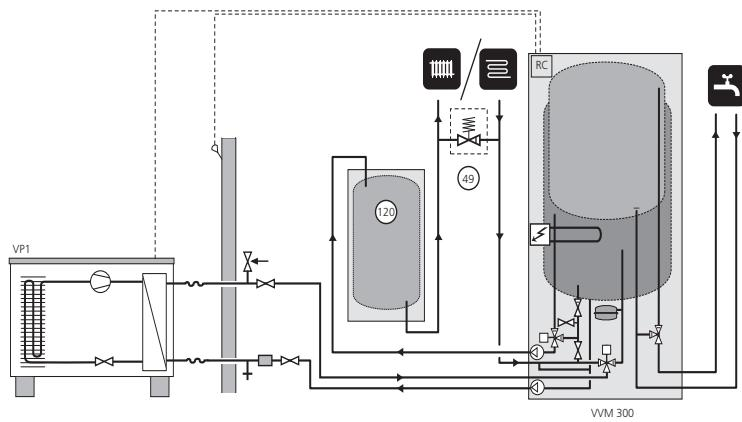
In cases where the system volume in the heating system is below 20 l/kW (heat pump output at 7/45°C) and/or the flow is choked uncontrolled, a UKV tank (120) is installed as a volume and flow increaser. Plug any connections that are not used. An automatic by-pass valve must be installed if there is a risk of potential 0-flow.
