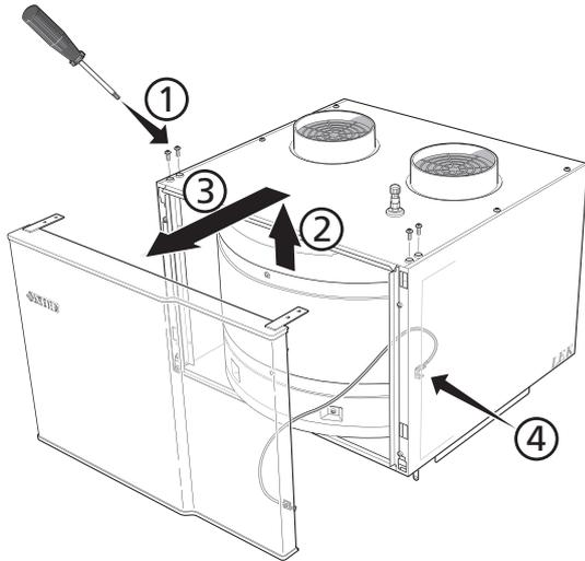
1. Slacken off the screws for the securing plate above F135.
