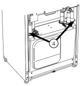
5. Remove the connection from the base card (AA2) using a screwdriver.
