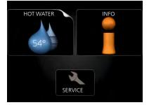
If the heat pump is set as slave a limited main menu is displayed because the majority of the settings for the system are made at the master heat pump.
