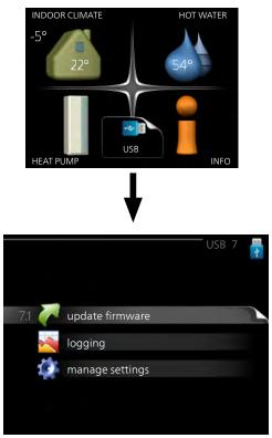
When a USB memory is connected, a new menu (menu 7) appears in the display.
