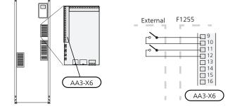
The example above uses the inputs AUX1 (X6:9-10) and AUX2 (X6:11-12) on the input board (AA3).
