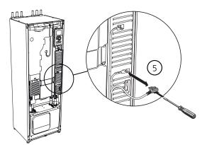
6. Disconnect the connectors (A) and (B) from the underside of the base card cabinet.
