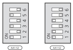
The image shows the dip-switch (AA1-S2) in the factory setting.
