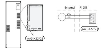
Activate the energy meter(s) in menu 5.2.4 and then set the desired value (energy per pulse) in menu 5.3.21.
