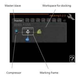
Master/slave: Select the heat pump for which the docking setting is to be made (if there is only one heat pump in the system, only master is displayed).
