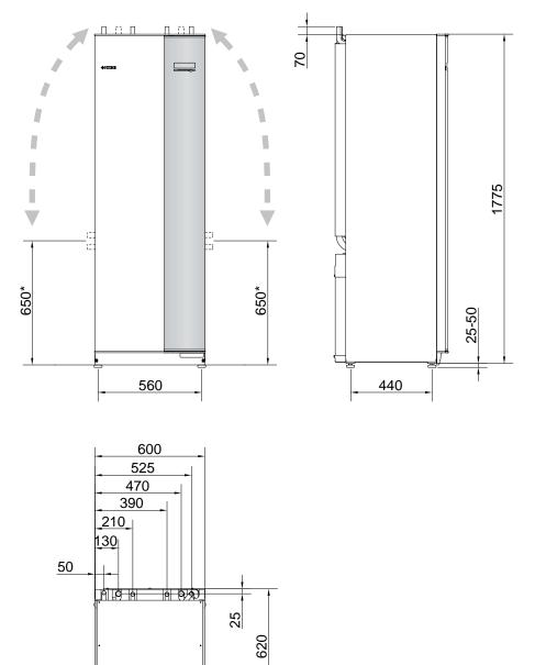
\* This dimension applies at 90° angle on the brine pipes (side connection). The dimension can vary approx. ±100 mm vertically as the brine pipes consist in part of flexible pipes.
