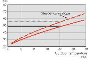
The optimum curve slope depends on the climate conditions in your location, whether the house has radiators, fan coils or underfloor heating and how well insulated the house is.
