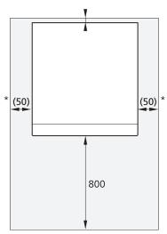
$^{*}$  A normal installation needs 300 – 400 mm (any side) for connection equipment, valves and electrical equipment.
