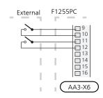
The example above uses the inputs AUX1 (X6:9-10) and AUX2 (X6:11-12) on the input board (AA3).
