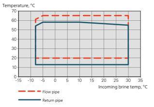
This diagram shows the working range above 75 % for F1255PC
