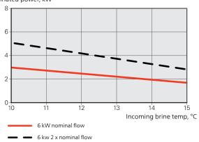
Passive cooling, 23 °C return temperature nominal flow brine/heating medium
