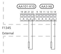
The example above uses the inputs AUX3 (AA3-X6:13-14) and AUX5 (AA101-X10:21-22) on the terminal block.
