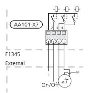
All additional heat can be blocked by connecting a potential-free switch function to AUX input on terminal block AA3-X6 and AA101-X10. The function must be activated in menu 5.4.
