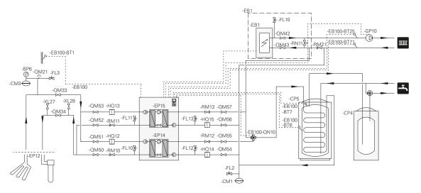
The heat pump (EB100) prioritises charging of hot water with a cooling module (EP14) via a reversing valve (EB100-QN10). When the water heater/accumulator tank (CP5) is fully charged, (EB100-QN10) switches to the heating circuit. When there is a demand for heat, cooling module (EP15) starts first. On greater demand, cooling module (EP14) also starts for heating operation.
