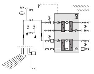
Install the brine pump (GP16) according to the circulation pump manual for connection of incoming brine (EP14-XL6) and (EP15-XL6) between the heat pump and shutoff valve (see image).
