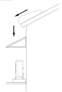
If there is a risk of snow slip from roof, a protective roof or cover must be erected to protect the heat pump, pipes and wiring.
