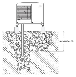
If the house has a cellar the stone caisson must be positioned so that condensation water does not affect the house. Otherwise the stone caisson can be positioned directly under the heat pump.
