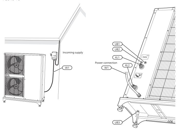
Incoming supply cable (W1) is enclosed and connected to terminal block X1 at the factory. Outside the heat pump there is approx. 1.8 m of cable available.
