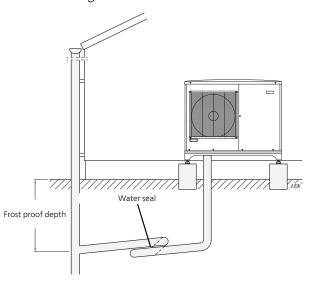
The outlet of the condensation water pipe must be at frost free depth.
