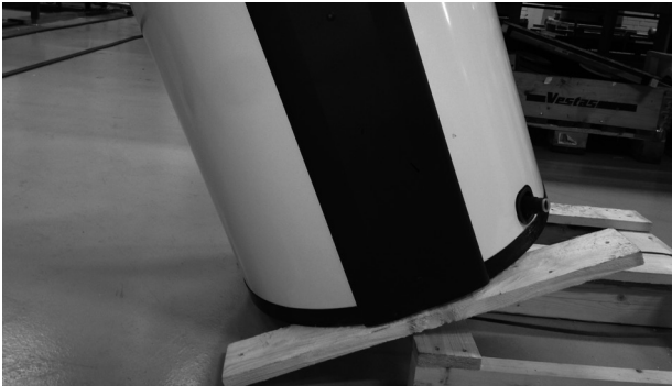
4. Removal of unit of from the pallet: a: Pull the unit carefully to one side. b: Tilt the unit to the same side together with the 2 pcs. of wood beneath.
