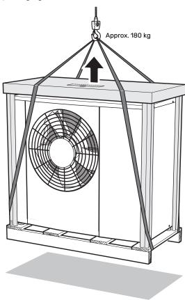
If S2125 needs to be transported across soft ground, such as a lawn, we recommend using a crane truck that can lift it to the installation location. When S2125 is lifted with a crane, the packaging must be untouched.
