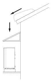
If there is a risk of snow slip from roof, a protective roof or cover must be erected to protect the heat pump, pipes and wiring.
