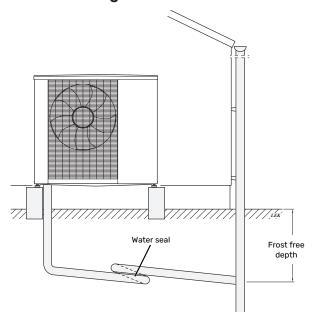
Route the pipe downward from the heat pump.
