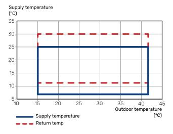
The working temperature of the heating medium is allowed to be lower for a short period, e.g. at start-up.
