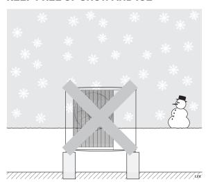
Prevent snow from building up and covering the grilles and drain holes on
