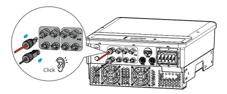
Seal the PV input terminals using waterproof covers when they are not to be used. Otherwise, the ingress protection rating will be influenced.
